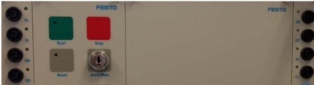
Figure 5. A typical FESTO Didactic Control Panel for HMI
